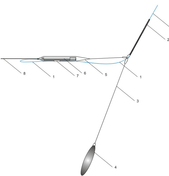
**Fig. 1 Composition of a towed undulating multi-parameter profiler.** 1 – towing cable, 2 – braided wire cable grip, 3 – rope, 4 – load, 5 – bridle, 6 – probe in plastic housing, 7 – connector, 8 – drag.
