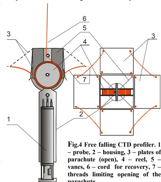
Fig.4 Free falling CTD profiler. 1 – probe, 2 – housing, 3 – plates of parachute (open), 4 – reel, 5 – vanes, 6 – cord for recovery, 7 – threads limiting opening of the parachute
