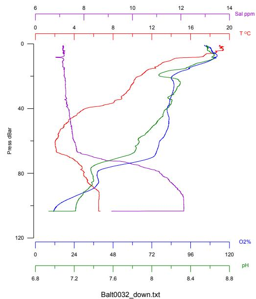
**Fig. 12** Vertical finestructure measured by free falling CTD
