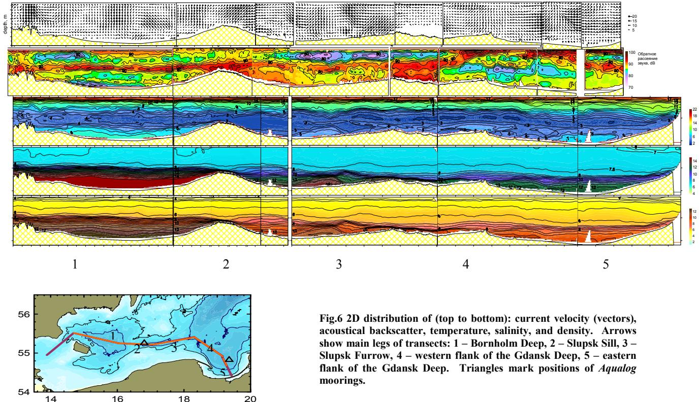
**Fig.6** 2D distribution of (top to bottom): current velocity (vectors), acoustical backscatter, temperature, salinity, and density. Arrows show main legs of transects: 1 – Bornholm Deep, 2 – Slupsk Sill, 3 – Slupsk Furrow, 4 – western flank of the Gdańsk Deep, 5 – eastern flank of the Gdańsk Deep. Triangles mark positions of *Aqualog* moorings.
