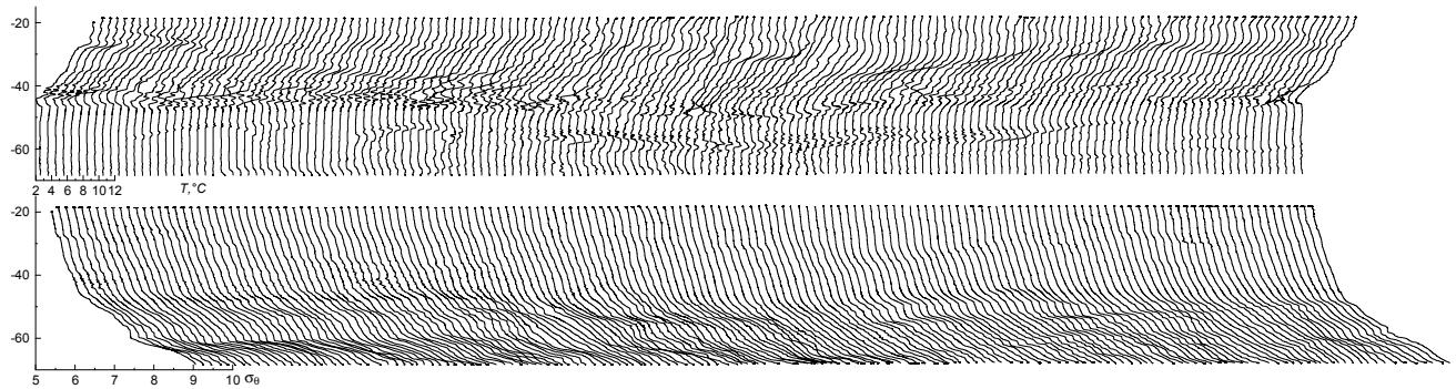
**Fig. 10** Time series of temperature and density finestructure profiles above the eastern slope of the Slupsk Sill
