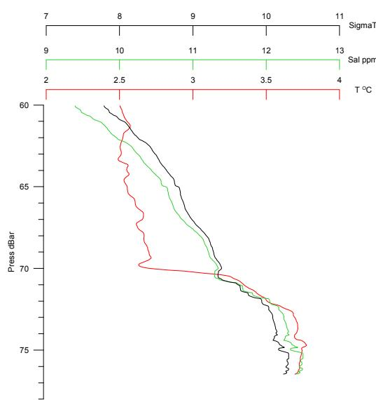
**Fig. 11** Vertical finestructure measured by free floating CTD
