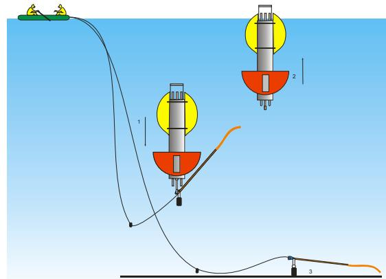
Fig.5 Sketch of a floating CTD profiler. 1 –sinking with ballast, 2 – floating up after releasing.
